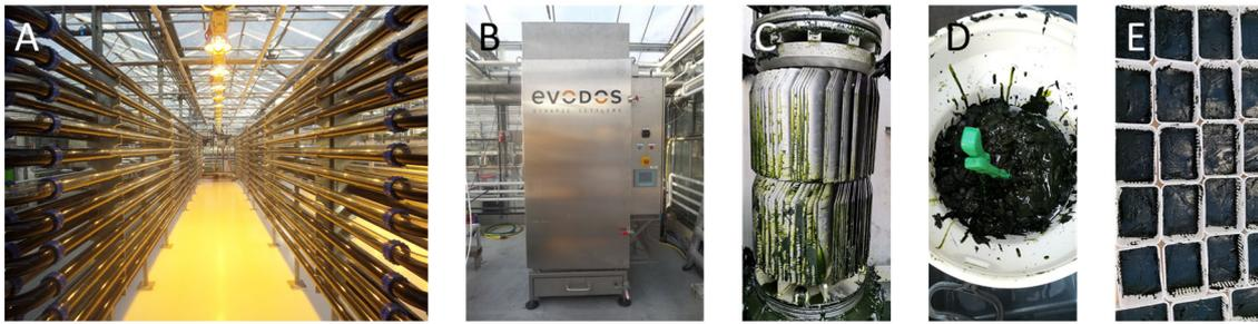
Figure 14– Representative scheme with pictures of the different steps involved in the harvesting and preparation of the biomass. A – large cultivation vessel, B – EVODOS centrifuge, C – Disk stack system of the EVOS centrifuge after being used with *Nannochloropsis*, D – collected biomass from the centrifuge, E – distribution of the algal biomass into smaller containers than will be frozen and later freeze-dried.
