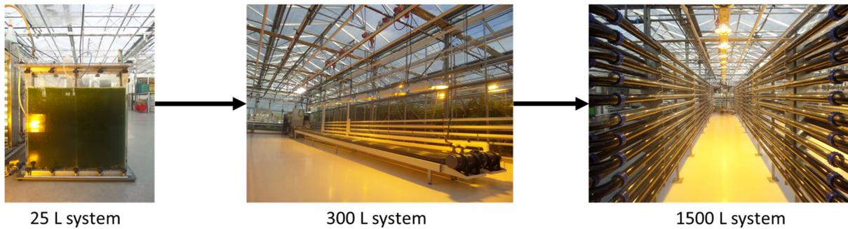
*Figure 2 – The scale up procedure of microalgal biomass for the fish feed trials on the different reactors available at AlgaePARC from the 25, to 300 to 1500 litre system. These systems will run during 2020 to achieve the necessary amount for the fishfeed trials.*
