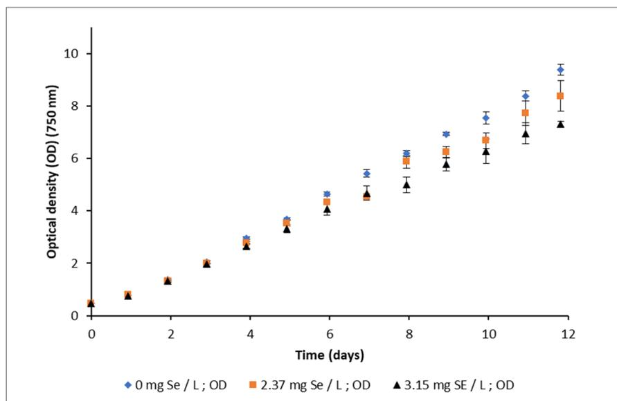
Figure 12 – OD during cell cultivation under different Se concentration 0, 2.37, 3.15 mg/L.
