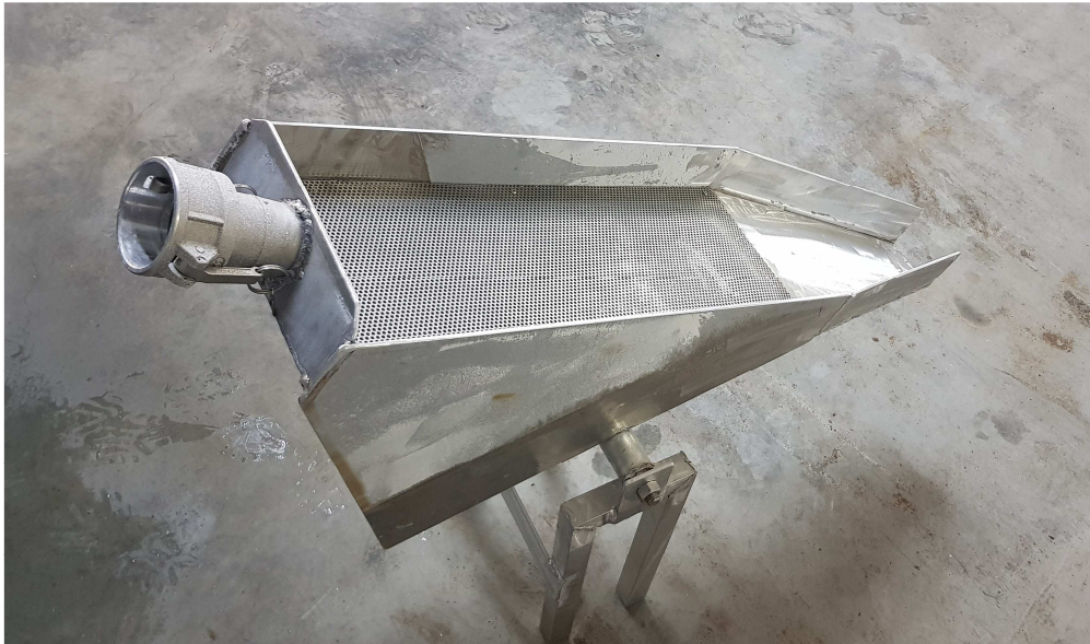
Figure 12: Device for separating fish mortalities from excess water
