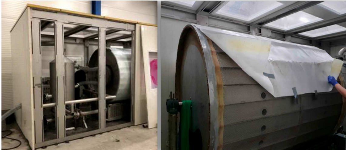
Figure 4.4.b – “S3 demonstration unit as produced by LS Optics AB. Right frame shows the details of the filter during change of filter cloth. Photo by Salten Havbrukspark AS (SHP)” (D2.1, Figure 6, Johansen et al. , 2019)
