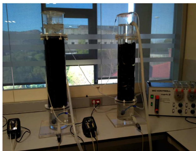
Figure 5.7 – “Built biofilter prototypes. Aeration is provided through an inlet at the bottom connected to an airstone” (Figure 4 in D2.4, Sousa et al. , 2019)
