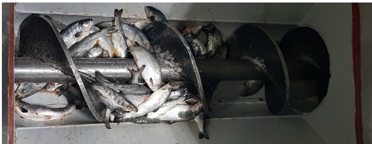
Figure 3.5 – “Mortalities in inlet buffer of Waister 15” (adapted from D2.6, Fig. 6, Baarset et al. , 2021)
