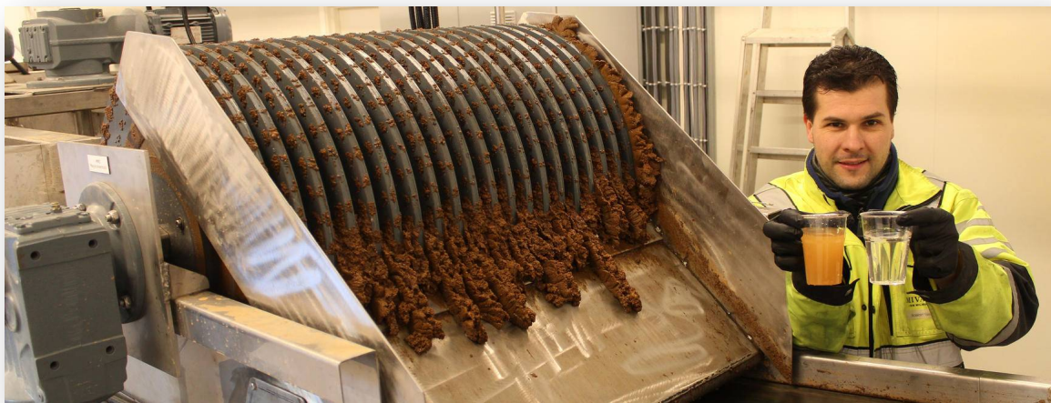
Figure 2. Magnetic particle separation (MPS) developed by Mivanor AS, and commercialised as MivaMag™. Photo with permission from Mivanor, showing water samples from the inlet and outlet of the MPS.
