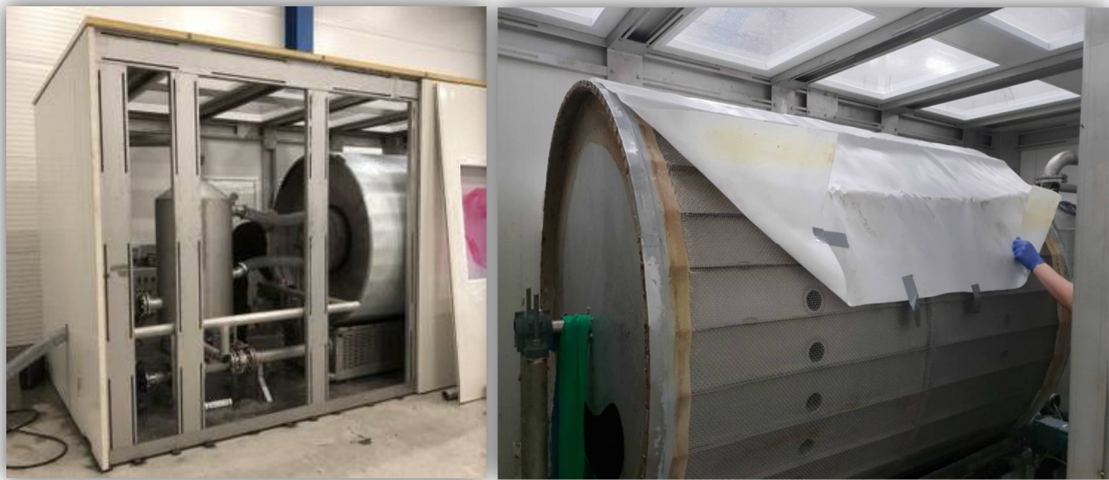
Figure 6. S3 demonstration unit as produced by LS Optics AB. Right frame show the details of the filter during change of filter cloth. Photo by Salten Havbrukspark AS.
