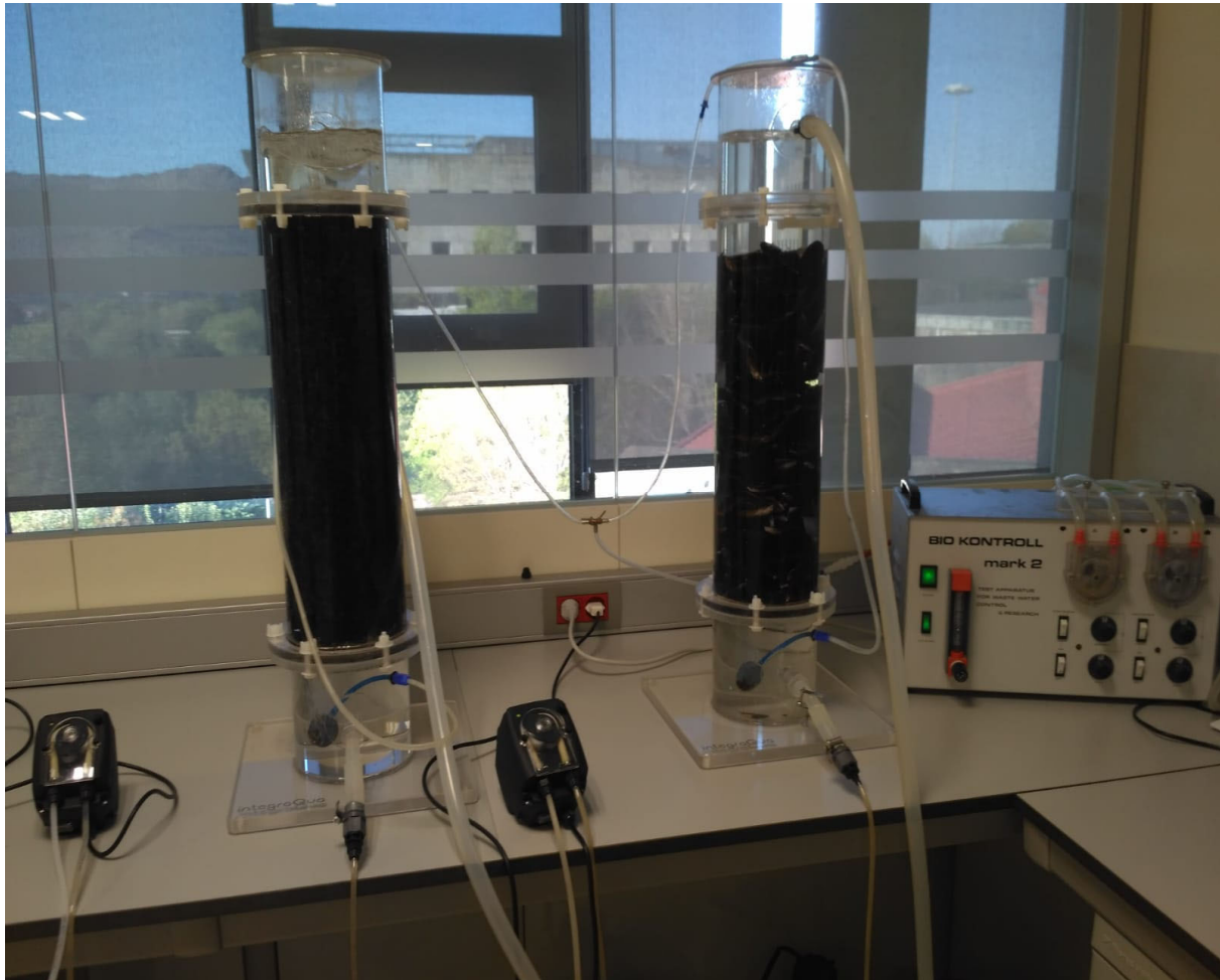
Figure 4. Built biofilter prototypes. Aeration is provided through an inlet at the bottom connected to an airstone.
