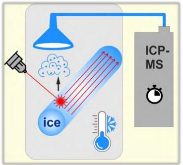
LA-ICP-MS is also a powerful technique for imaging the 2D impurity distribution of solid samples, an application which still remains to be fully exploited for ice cores.
